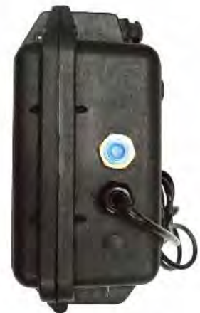
Right side showing power cable and sample air input point
