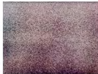
Condition C Blasted to Sa2
