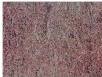
Condition B Blasted to Sa2
