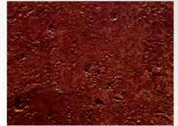
Condition D Blasted to Sa1
