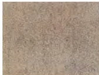
Condition B Blasted to Sa2.5
