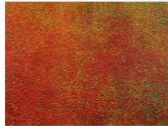
Condition C Blasted to Sa1
