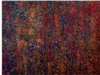
Condition B Blasted to Sa1
