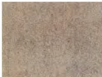
Condition B Blasted to Sa2.5
