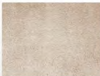
Condition B Blasted to Sa3
