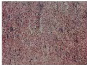
Condition B Blasted to Sa2
